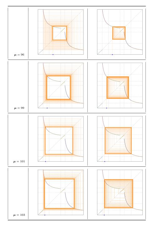
TABLE 7. The plot of the projective map  $\varphi_{\mu} : [0,2] \rightarrow [0,2]$ , where the blue dot in int  $(J_k)$  is the initial condition, whith k = 2, 3 for  $\mu = 96$ , and  $\mu = 99, 101, 103$ , respectively, and the orange lines follows its 100 iterates by  $\varphi_{\mu}$ .
